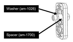
3. Place two 10-32 x 1500 screws (am-1047) through the 2x4 as shown and add a #10 washer (am-1026) on each.
