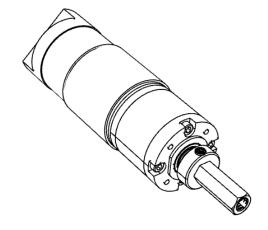
18. Install one NeveRest Orbital gearmotor to the motor mount plate using four M3-8mm patched screws (am-1500).
