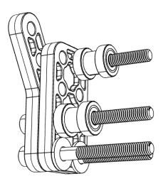
12. Place one 2x4 plate (am-5006\_2x4) and one 150° angle bracket (am-5010\_150) onto the four screws. Loosely secure with four 10-32 Nylock nuts (am-1063).
