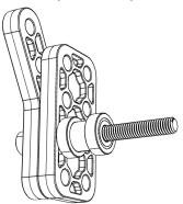
9. Place one 10-32 x 1500 screw (am-1047) through the plate assembly and add one #10 washer (am-1026) to the screw.
