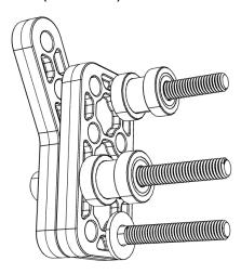
11. Place the bottom two screws in the assembly through the end holes in one 0.5 x 0.5 Robits Tube. Add a #10 washer (am-1026) next to the tube onto each of the two screws.
