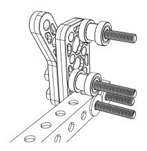
8. Install two bearings (am-4724) with a  $\frac{1}{4}$ " screw spacer (am-1700) between them onto one 10-32 x 1500 screw (am-1047) in the plate assembly as shown.
