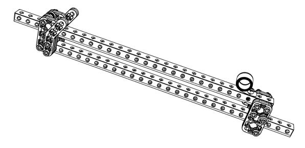
14. Place one 1" screw spacer (am-1696) between two #10 washers (am-1026). This will go inside the spring coil.
