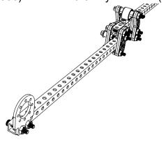
15. Place one 10-32 x 2000 screw (am-1049) through the washers and spacer and secure with one 10-32 Nylock nut (am-1063).
