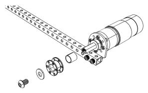
20. Tie a length of string from the ½" screw spacer on the extension to the spool.
