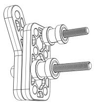
10. Place one 10-32 x 2000 screw (am-1049) through the plate assembly and add one #10 washer (am-1026) to the screw.
