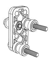
4. Place the top two screws in the assembly through the end holes on one 0.5 x 0.5 Robits Tube. Add a #10 washer (am-1026) next to the tube onto each of the two screws.
