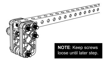
2. Add two bearings (am-4724) with a  $\frac{1}{4}$ " screw spacer (am-1700) between them onto one 10-32 x 1500 screw (am-1047) to create a roller shaft as shown.
