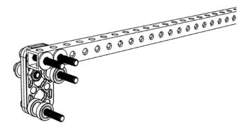
6. Fasten one spring (am-4666) to the next hole on the tube using one 10-32 x 0750 screw (am-1047) and one 10-32 Nylock nut (am-1063).
