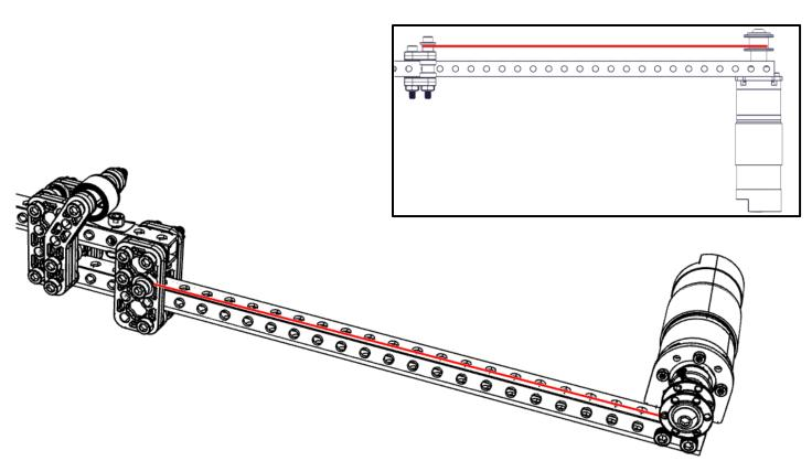
The Spring Extend Assembly is complete! When the motor turns the string will wrap around the spool and extend the spring.
