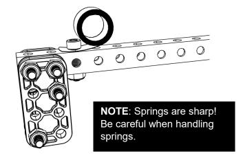
7. Align one 150° angle bracket (am-5010\_150) to one 2x4 plate (am-5006\_2x4) as shown. Install two bearings (am-4724) with a  $\frac{1}{4}$ " screw spacer (am-1700) between onto one 10-32 x 2000 screw (am-1049).
