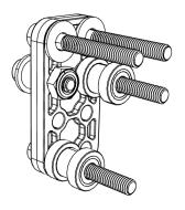
5. Place one 2x4 plate (am-5006\_2x4) onto the four screws and loosely secure with four 10-32 Nylock nuts (am-1063).
