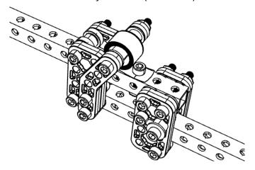
17. Place one 6mm to 375 Hex adapter (am-3444) on the motor shaft. Make sure to secure by tightening the provided 10-32 set screw.
