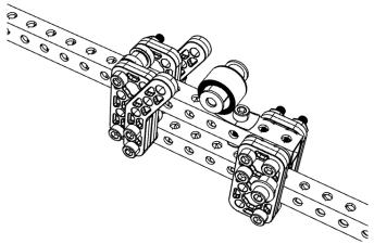
16. Install one motor mount (am-5012) to the end of the 0.5 x 0.5 tube without the spring. Attach with two 10-32 x 1000 screws (am-1056) and two 10-32 nylock nuts (am-1063).
